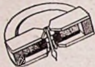
Held in position by magnetic attraction, without restriction by mechanical contact.
